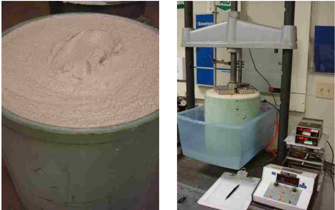
Figure 4.1. Slurry Consolidation (98.5% Kaolin : 1.5% EPS)
