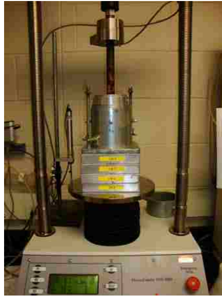
Figure 4.3. Static Undercompaction of Specimens
